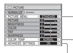
Press the left ◀ or right ▶ button to select "ON". Press the down ▼ button to enter ADVANCED SETTINGS mode. ADVANCED SETTINGS ON Enables fine picture adjustment at a professional level (see next page).
